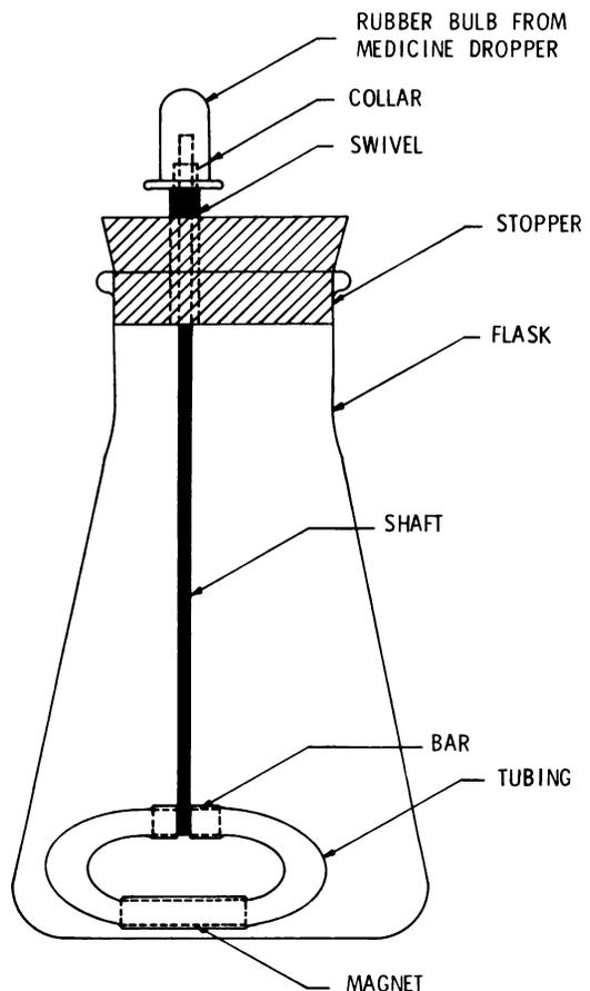
FIG. 1. Stirrer hanging in flask.
