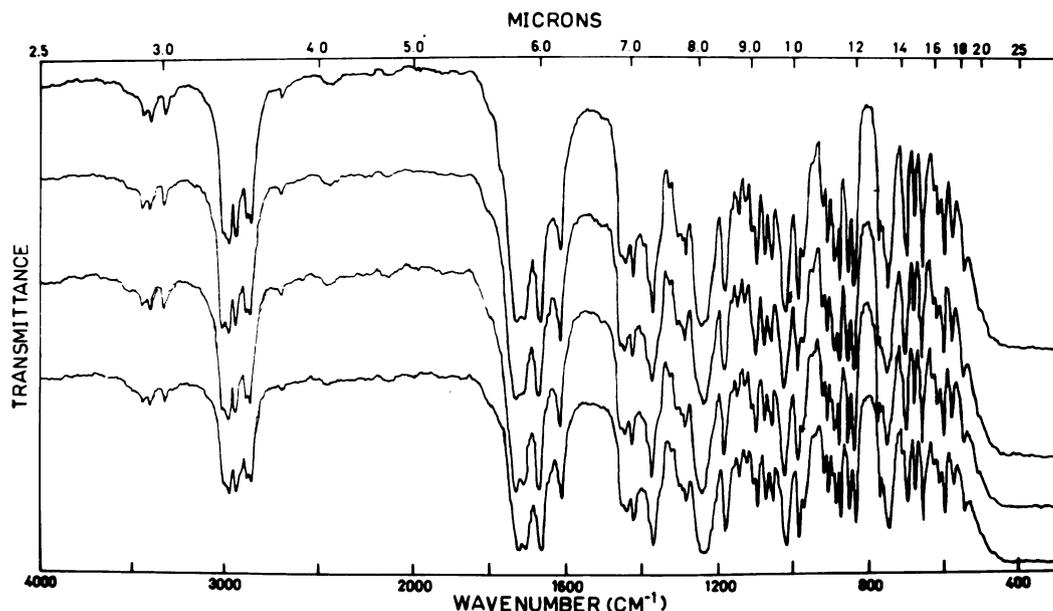
FIG. 2. Infrared spectra of PR toxin isolated from different *P. roqueforti* strains. The samples were dissolved in  $\text{CHCl}_3$  and deposited on demountable cells as thin film by solvent evaporation. Spectra from the top to the bottom are samples from strains ATCC 6987, ATCC 6989, ATCC 9295, and ATCC 10110.
