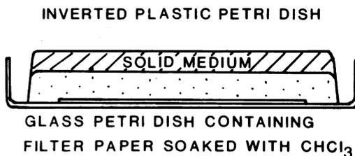
FIG. 1. Device for killing bacteria in plastic petri dishes by exposure to chloroform vapors.
