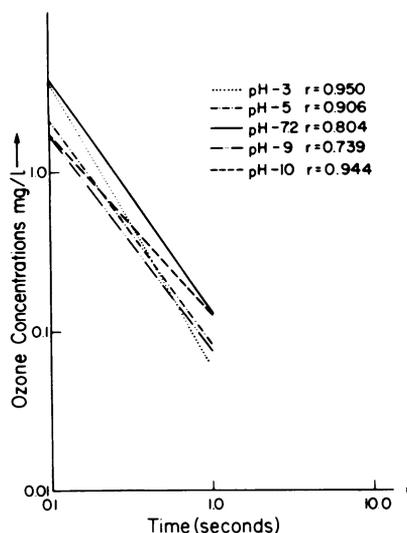
FIG. 3. Effect of pH on time-concentration relationship for 95% inactivation of poliovirus type 1 by ozone (log-log scale).  $r$ , Correlation coefficient.
