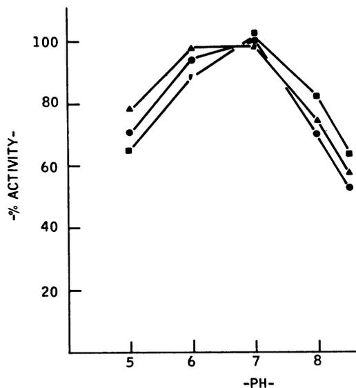
FIG. 7. Effect of pH on the production of acetone from oxidation of *n*-propane by cell suspensions of methylotrophs. The products were identified and estimated by gas chromatography. Symbols are as in Fig. 1. 100% activity = 1.5, 1.4, and 1.2  $\mu\text{mol}$  of acetone produced/h per 5.0 mg of protein concentration in cell suspensions of *Methylosinus* sp. (CRL-15), *Methylobacterium* sp. (CRL-26), and *Methylococcus capsulatus* (Texas), respectively.
