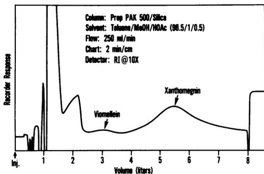
FIG. 1. Preparative high-pressure liquid chromatogram of xanthomegnin purification.
