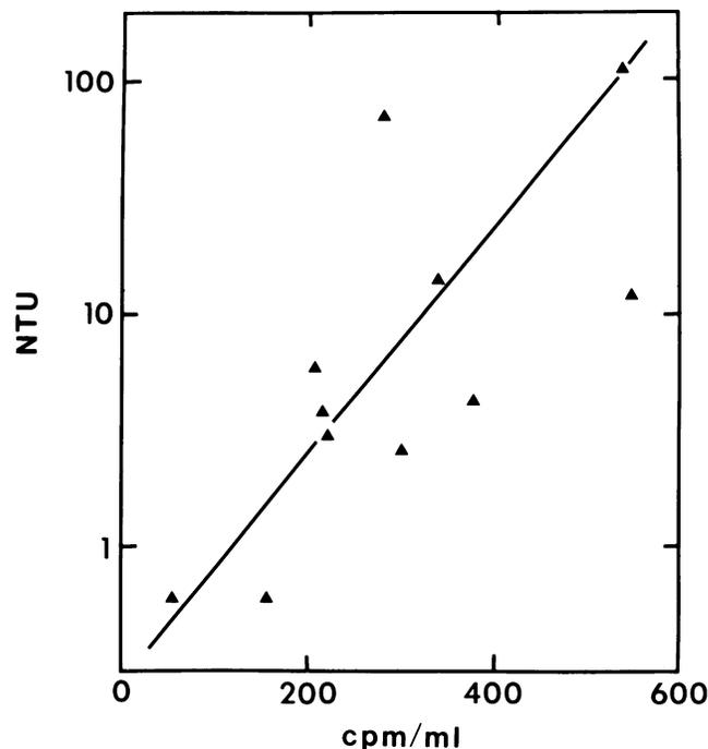
FIG. 3. Effect of turbidity (NTU) of different waters on adhesion of radioactively labeled polioviruses to container walls. An average of 1.027 cpm of [ $^3\text{H}$ ]uridine-labeled poliovirus per ml was seeded into different waters, and the flasks (Pyrex glass) were held stationary during incubation. Recoverable radioactivity shown in this plot was determined after 1 day at 26°C.
