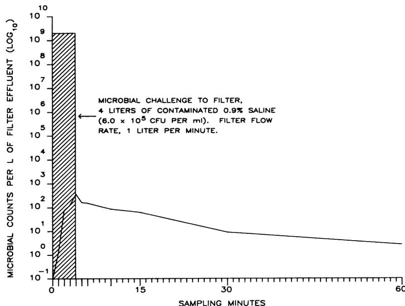
FIG. 5. *P. pickettii* challenge of a 0.2- $\mu$ m absolute cartridge filter.
