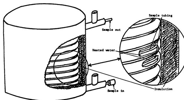
FIG. 1. Tube-in-tube flowthrough pasteurization device.
