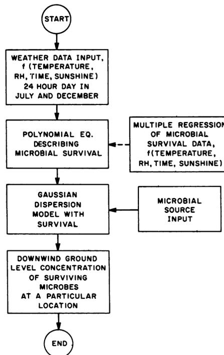
FIG. 2. Flow diagram of the dispersion model algorithm.
