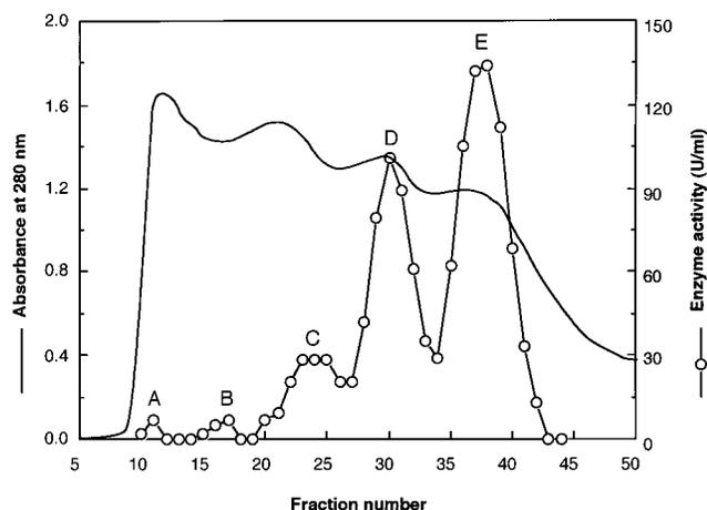
FIG. 1. Gel filtration of *A. caviae* ME-1 xylanases on Sephadex G-75. The column (84 by 2.6 cm) was equilibrated and eluted with 0.2 M NaCl in 20 mM potassium phosphate buffer (pH 6.8) at a flow rate of 30 ml/h, and 7 ml of the fractions was collected. Peaks A, B, C, D, and E correspond to xylanases V, IV, III, II, and I, respectively. —,  $A_{280}$ ; ○, xylanase activity.
