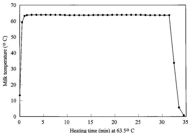
FIG. 1. Heating-cooling curve for holder pasteurization at 63.5°C.
