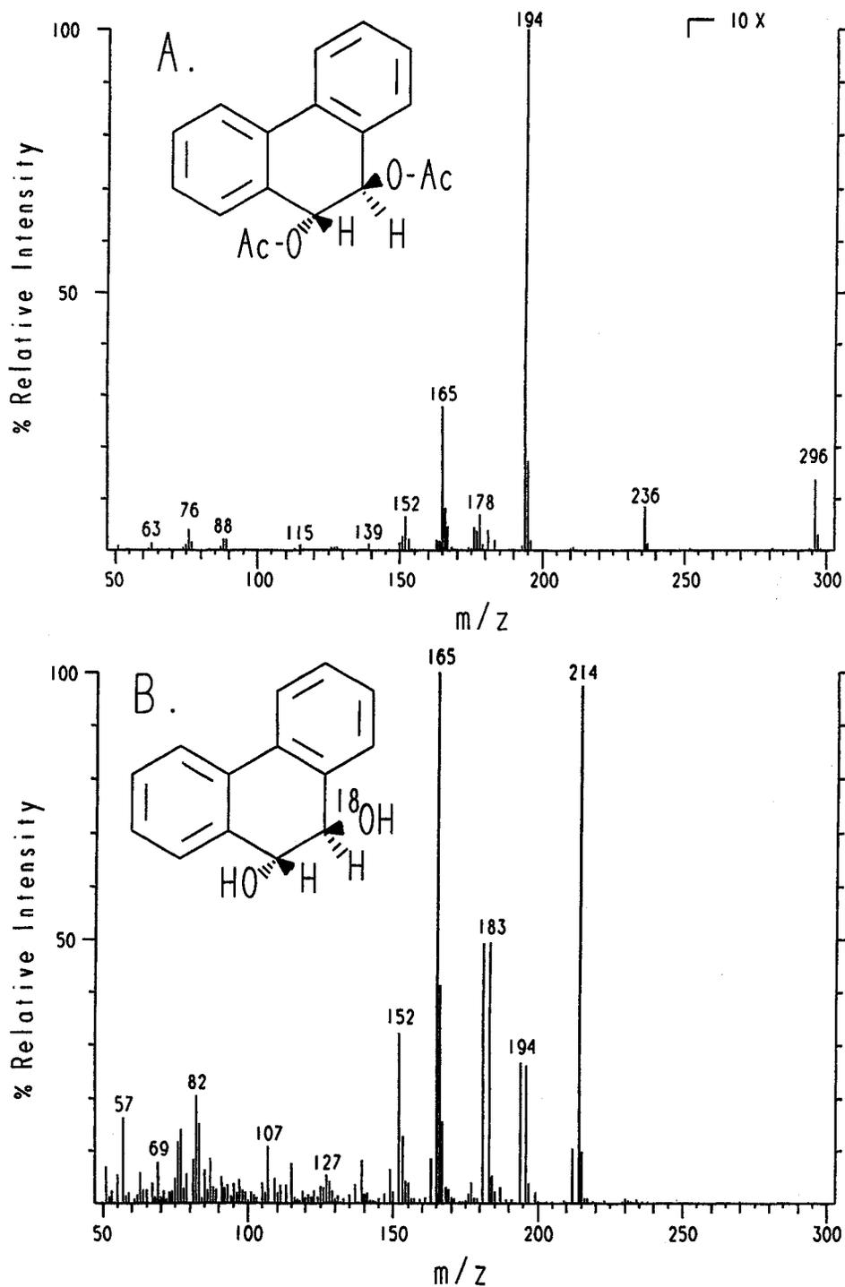
FIG. 3. (A) Mass spectrum of the acetylated derivative of phenanthrene *trans*-9,10-dihydrodiol produced from phenanthrene by *P. ostreatus*. (B) Mass spectrum of phenanthrene *trans*-9,10-dihydrodiol formed in the  $^{18}\text{O}_2$  incorporation experiment.
