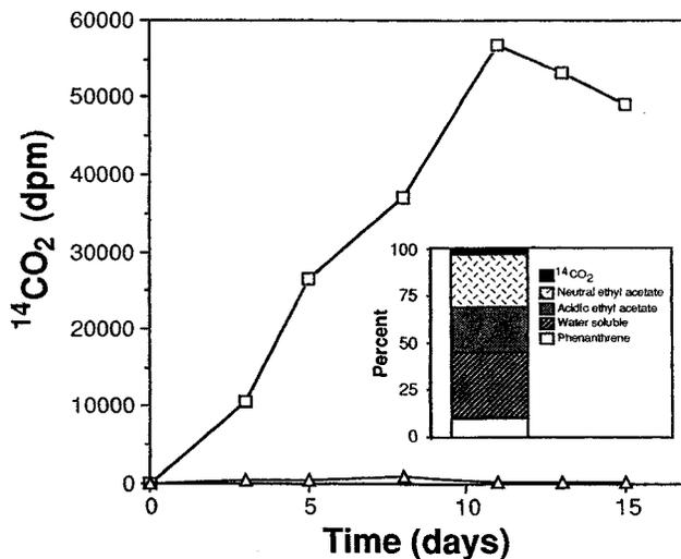
FIG. 1. Mineralization of [9,10-<sup>14</sup>C]phenanthrene by *P. ostreatus* (□) and control incubation of phenanthrene in BRM without the fungus (△). The insert represents the distribution of phenanthrene mineralization. The mass balance represents the percent recovery of radioactivity initially added.
