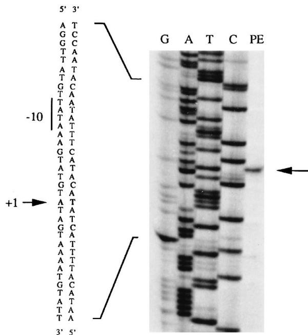
FIG. 3. Primer extension analysis. An oligonucleotide complementary to the *pta* sequence was hybridized to RNA isolated from an exponential-phase culture of *C. acetobutylicum* and extended by reverse transcriptase. Lane PE, the primer extension product; lanes G, A, T, and C, sequencing reaction products, with the same oligonucleotide as the primer and recombinant plasmid pUC-PTAK as the template. Arrows indicate the position of the transcriptional start site.
