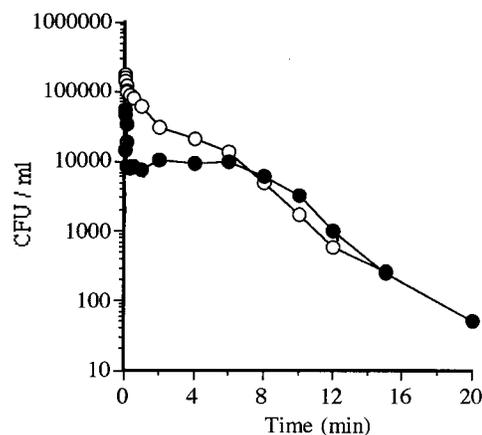
FIG. 4. Survival curves of *B. coagulans* at  $108.5^{\circ}\text{C}$  in McIlvaine buffer (pH 7) before (●) and after (○) a sublethal heat shock for 3.5 h at  $80^{\circ}\text{C}$  in distilled deionized water.
