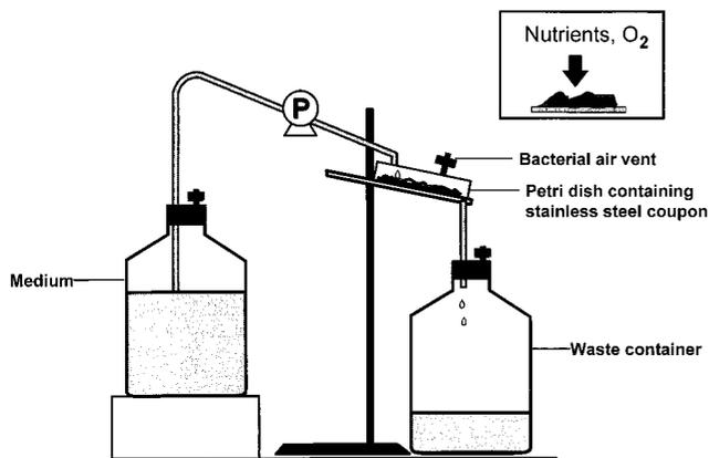
FIG. 1. Schematic diagram of our drip-flow biofilm reactor.
