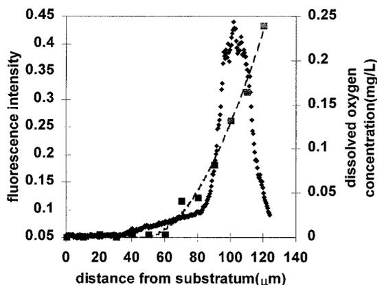
FIG. 5. Correlation of the dissolved-oxygen profile with the image analysis result of APase expression under aerobic conditions.  $\blacklozenge$ , APase activity;  $\blacksquare$ , dissolved oxygen;  $-\cdot-$ , trend line representing dissolved-oxygen concentration.
