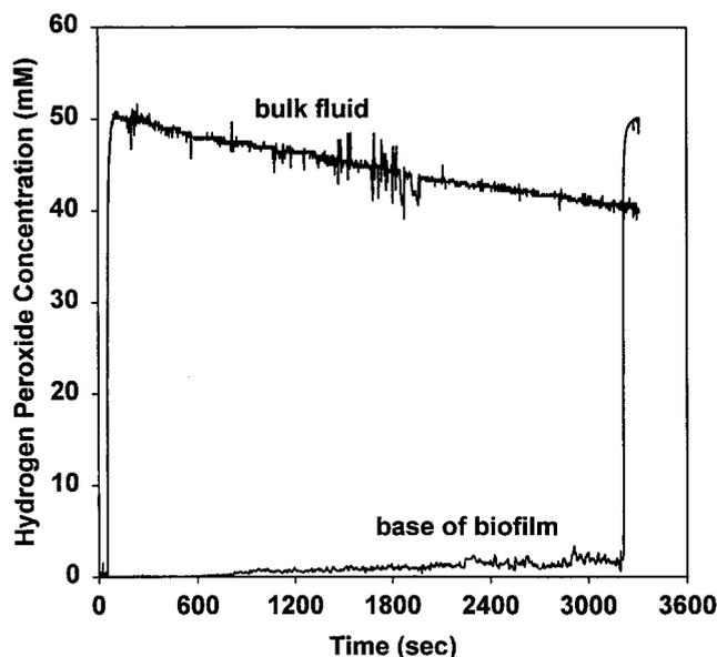
FIG. 1. Failure of  $H_2O_2$  to penetrate a wild-type *P. aeruginosa* biofilm. The microelectrode corresponding to the data set designated base of biofilm was withdrawn from the biofilm into the bulk fluid after approximately 3,200 s. The spike in the signal at this time indicated that the electrode was still sensitive to  $H_2O_2$ .
