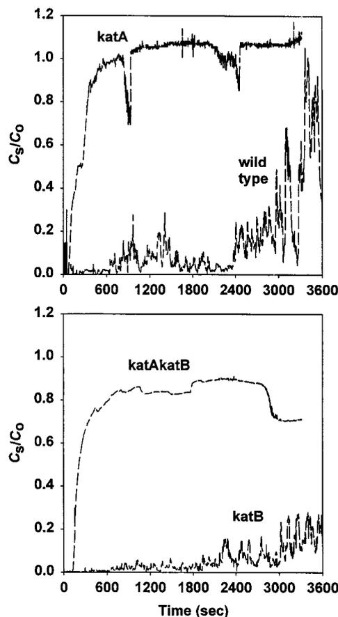
FIG. 2. Comparison of  $H_2O_2$  penetration into wild-type and catalase mutant *P. aeruginosa* biofilms. The ratio plotted on the y axis,  $C_s/C_o$ , is the concentration of hydrogen peroxide measured within approximately 10  $\mu\text{m}$  of the substratum divided by the concentration of hydrogen peroxide in the bulk fluid.
