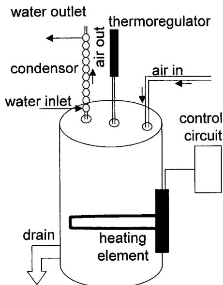
FIG. 1. Bioreactor schematic.
