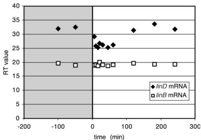
FIG. 3. Real-time PCR analysis of *linB* and *linD* gene expression in *S. paucimobilis* B90A. The mRNAs were purified from the induction experiment with  $\gamma$ -HCH (7 mg/liter) as described in the legend of Fig. 2. The time sequence is that described in the legend of Fig. 2. The y axis shows the threshold cycle number during which exponential amplification starts.
