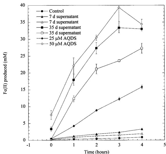
FIG. 3. Fe(III)-oxide reduction by *G. sulfurreducens* resting cell suspensions incubated with supernatants from *G. fermentans* fuel cells. Effects of supernatants from two 7-day-old fuel cells ( $\Delta$ ,  $\blacktriangle$ ) and two 35-day-old fuel cells ( $\square$ ,  $\blacksquare$ ) are shown, with the effects of 25  $\mu\text{M}$  ( $\blacklozenge$ ) and 50  $\mu\text{M}$  ( $\diamond$ ) AQDS shown for comparison.
