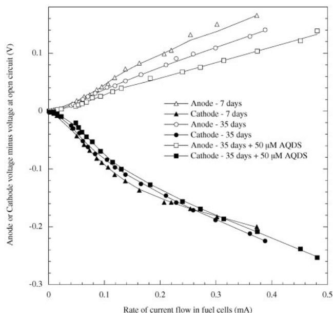
FIG. 4. Overvoltages for anodes and cathodes in a representative *G. fermentans* fuel cell over a range of current densities. Characteristics were measured 7 days after medium replacement ( $\Delta$ ,  $\blacktriangle$ ), in the same fuel cell 35 days after medium replacement ( $\circ$ ,  $\bullet$ ), and with 50  $\mu\text{M}$  AQDS addition 1 day later ( $\square$ ,  $\blacksquare$ ). Values closer to zero as the rate of current flow increases indicate improvements in operating cell voltage.
