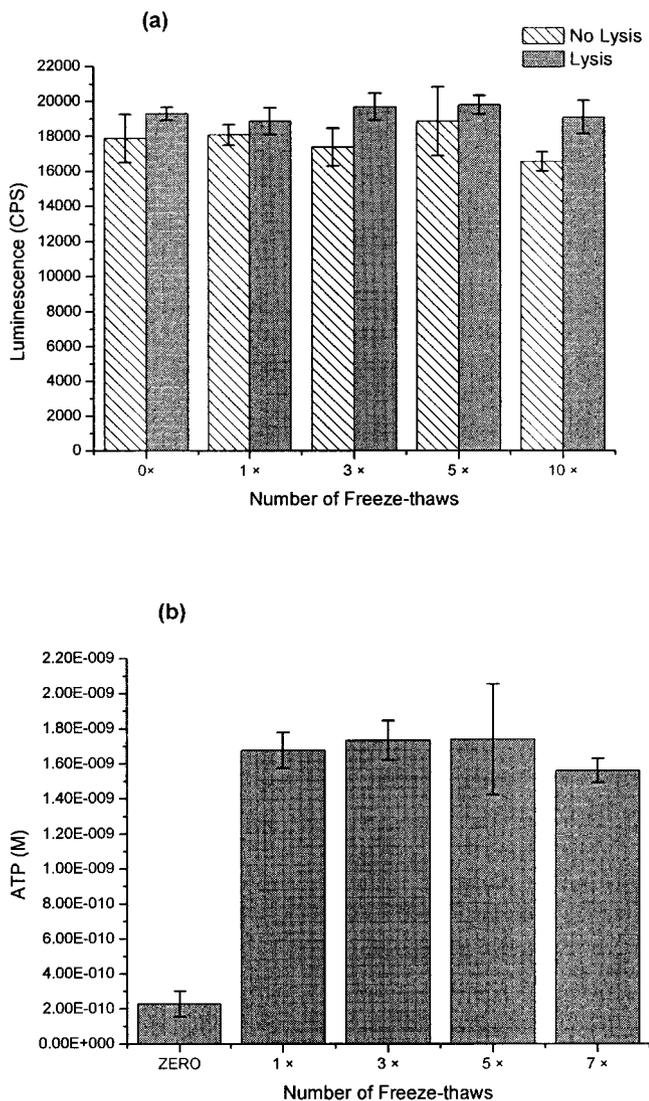
FIG. 3. a. Effect of freeze-thaws on ATP as quantified by bioluminescence using the luciferin-luciferase reaction ( $n = 3$ ). Error bars indicate standard deviations. b. Effect of freeze-thaws on ATP extracted from 10,000 *Cryptosporidium* oocysts ( $n = 3$ ). Error bars indicate standard deviations.
