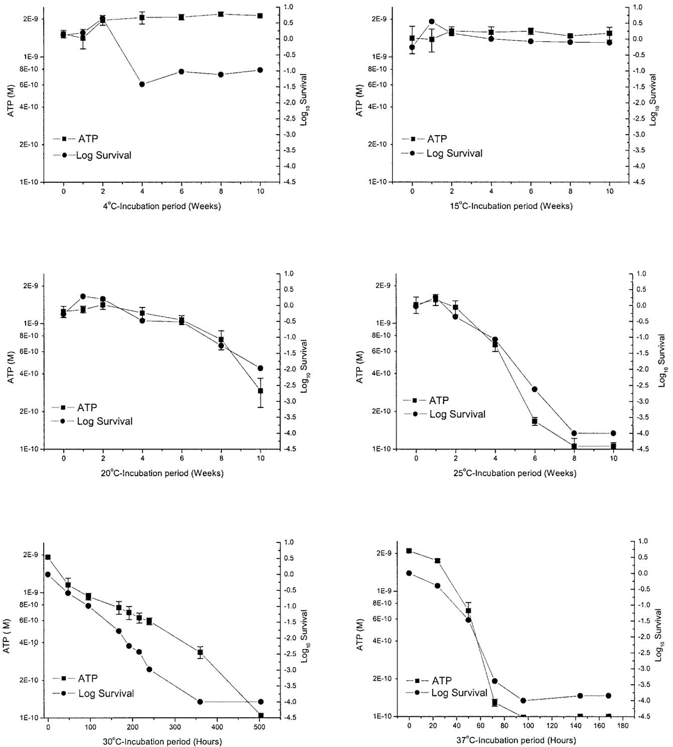
FIG. 5. Relationship between oocyst infectivity and oocyst ATP for 10,000 *Cryptosporidium* oocysts incubated in reagent-grade MilliQ water at incubation temperatures of 4, 15, 20, 25, 30, and 37°C. For cell culture results, survival at 4°C was calculated using the 4°C time zero sample as a control. For other temperatures, the corresponding 4°C sample was used as a control for each time point. Error bars indicate the standard deviations for ATP measurements.
