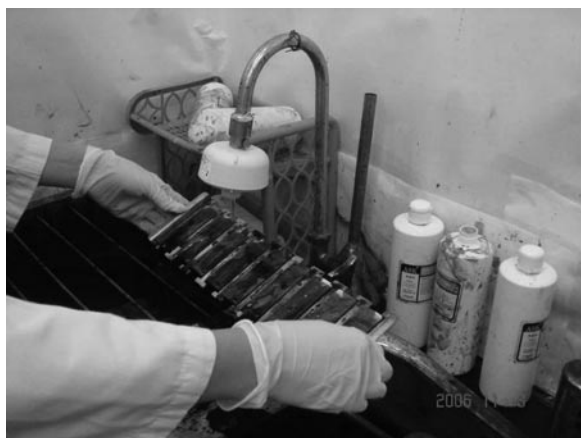
FIG. 1. A point-of-use water filter attached to the water outlet for acid-fast staining procedures.
