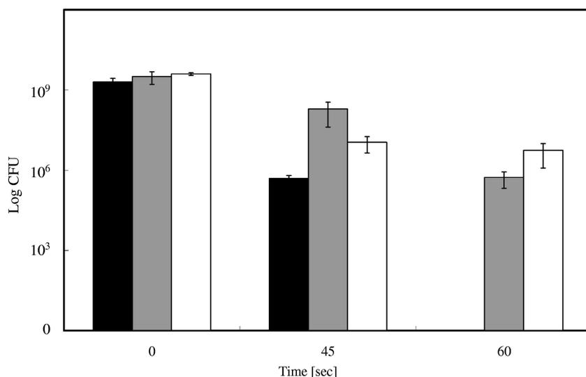
FIG. 3. Protective effects of metal chelators for survival of *E. coli* on copper surfaces. Cells were treated as described in the legend for Fig. 1 except samples were withdrawn only after 0, 45, and 60 s. Cells were mixed with  $\text{Cu(II)}$  chelator EDTA (gray bars),  $\text{Cu(I)}$  chelator BCS (white bars), or no chelator (black bars) prior to application onto copper surfaces. Shown are averages with standard deviations (error bars) from three independent experiments.
