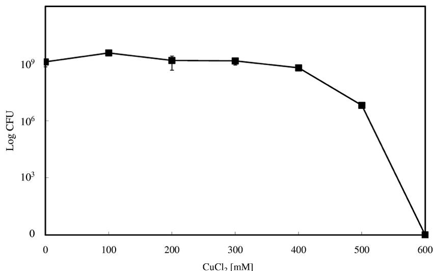
FIG. 2. Killing of *E. coli* by aqueous  $\text{CuCl}_2$ . Cells of *E. coli* wild-type strain W3110 were diluted in different  $\text{CuCl}_2$  solutions and incubated at  $23^\circ\text{C}$  for 1 min. Samples were diluted and plated on LB agar. Surviving cells were counted as CFU after 16 h at  $37^\circ\text{C}$ . Shown are averages with standard deviations (error bars) from three independent experiments.
