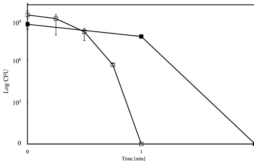
FIG. 6. Survival of *E. coli* strains on copper surfaces under anaerobiosis. Cells of *E. coli* W3110 were treated as described in the legend for Fig. 1 except that exposure to copper surfaces was conducted under an  $N_2$  atmosphere (filled symbols) or air (open symbols). Error bars indicate standard deviations.
