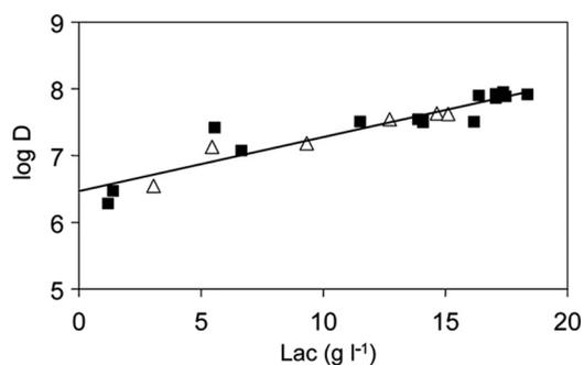
FIG. 3. Relationship between the logarithm of dead cell counts measured by flow cytometry (D, cells  $\text{ml}^{-1}$ ) and dissociated lactate concentration in the culture medium (Lac, g  $\text{liter}^{-1}$ ), during fermentations performed at pH 6 (■) and pH 5 (△).
