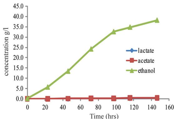
FIG. 5. High ethanol titer using the *C. thermocellum* evolutionarily (ev) engineered version of the  $\Delta hpt \Delta ldh \Delta pta$  strain and in a *T. saccharolyticum* ALK2 coculture. A batch reactor with continuous stirring set at 300 rpm with an initial pH of 6.3 and 92.2 g/liter Avicel was maintained at 55°C. Data represent a single fermentation sampled over the course of 146 h.
