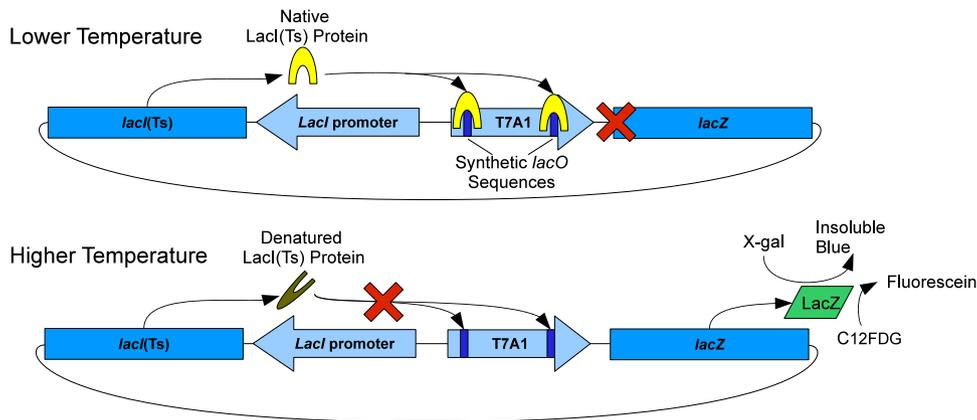
FIG. 1. Diagram of a LacI(Ts)-controlled thermometric system. At lower temperatures, the constitutively expressed LacI(Ts) can bind to the synthetic *lacO* sites engineered into the T7A1 promoter, preventing expression of LacZ. As temperatures increase, 2° and 3° structural changes in the LacI(Ts) molecules result in decreased binding at the *lacO* sites, leading to increasing expression of LacZ. LacZ expression can be detected using colorimetric (X-gal) or fluorometric (C12FDG) substrates.
