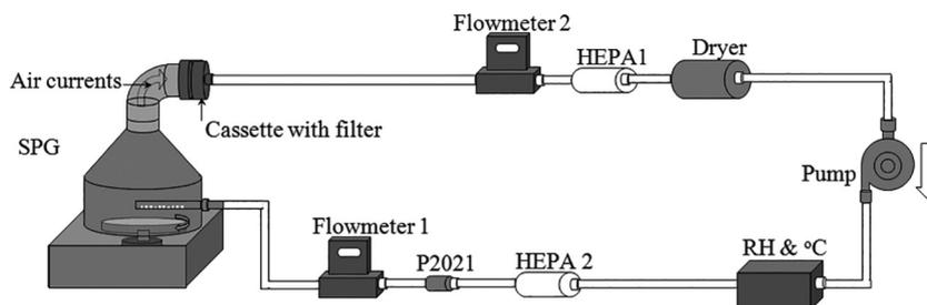
**FIG 2** Experimental setup. The generator (SPG) with mounted cassette is connected to the system setup. Flowmeters 1 and 2 measure the airflows at the inlet and outlet of the generator, respectively. HEPA 1 and HEPA 2 filter the airflows from the outlet and to the inlet, respectively. The dryer (in-line tube containing silica gel) maintains a constant relative humidity in the air at the inlet, and the in-line P2021 ionizer reduces electrostatic charges.
